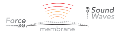
With Edge Motion™ technology, pressure along the side generates perpendicular sound waves
